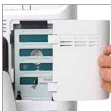
Service Access for Replacing HDD
